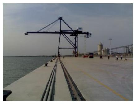
The first of 7 STS cranes of SITV in place at the newly installed Crane Rail System from MHE-Demag Vietnam and Gantrail.
